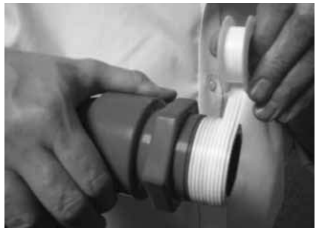
Illustration shows use of the inner socket of the reducer.
